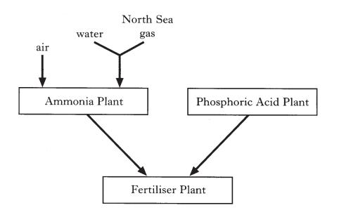
(a) Air and water are used as raw materials because they contain the elements needed to make ammonia.
